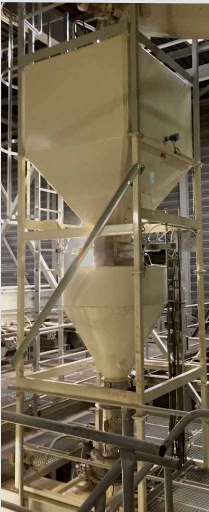
Post pelleting application MVS Coating system for : - Fat, Soya oil, fatty acid. - Enzymes, phytase. - Probiotics.
